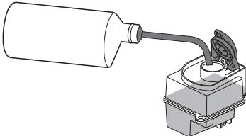
**Fill the tank completely with fuel. Use only 20% to 25% Nitro content fuel. Use high quality branded model car fuel only. Using the incorrect fuels could damage the engine and void the warranty.**
