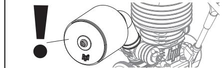
**Engine must always have air filter installed before and during engine operation!**
