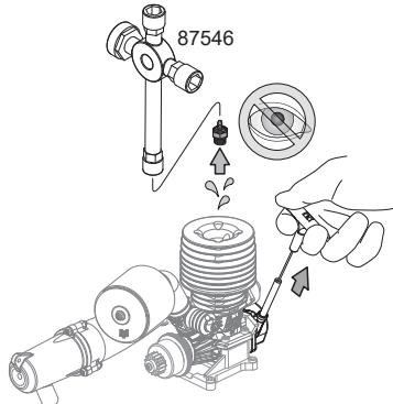
If there is too much fuel in the cylinder, the engine will not start. Follow the steps below to remove excess fuel from the cylinder.
