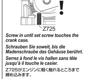
Screw in until set screw touches the crank case.
