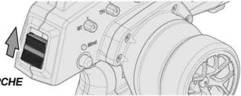
3 Press and hold the receiver setup button, then turn the power switch to the ON position. The receiver LED will flash quickly. Release the setup button after 1 second.
