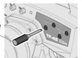
End point adjustments allow you to set the limits of steering and throttle.
