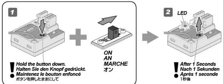
4 Press and hold the binding button on the transmitter for 1 second until the LED on the receiver is continuously lit.
