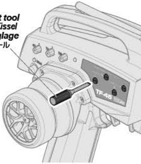
End point adjustments allow you to set the limits of steering and throttle.
