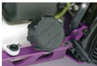
Fuel tank is held by quick release clips. The cap indicates the required fuel/oil mix
