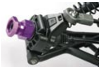
The Baja features hubs that bolt together and gaiters on the driveshafts
