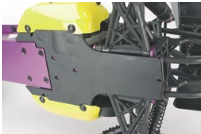
A moulded section covers the screws that holds the rear suspension and gearbox in place
