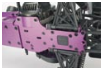
The chassis comes in two parts with a moulded cover plate for the rear section - see right
