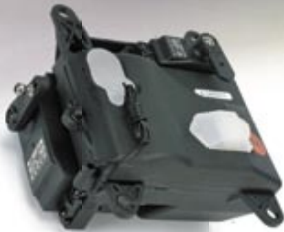
Above: The radio unit can be removed containing the servos, receiver and 2000mAh battery pack
