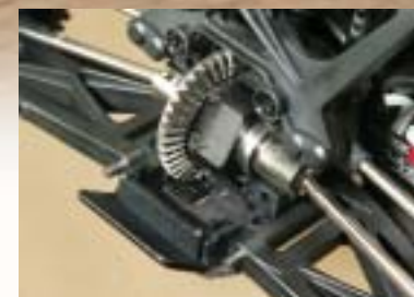
With the diff case removed, the straight-cut bevel gear and plated steel outdrives are visible. Inside the cases are hardened-steel gears that will deal with the abuse the powerful engine subjects the drivetrain to.
