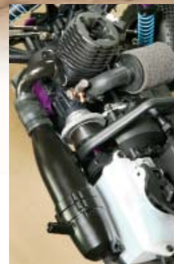
The cast-aluminum, black-coated tuned pipe is a major upgrade of the MT2 platform. It took me a little while to get used to the new pipe, and I have burn marks to prove it, but the chamber does let the power roar.
