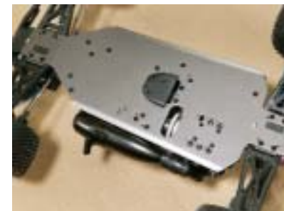
The hard-coated gray chassis features flared edges that strengthen it. The screw holes are countersunk, and notches in the chassis let the gear cases sit low. Check out the gear skid with its molded flame design. It protects the spur gear but gives it room to eject debris.
