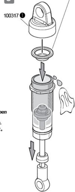
! If shock shaft is bent, replace shock shaft and silicone O-rings.
