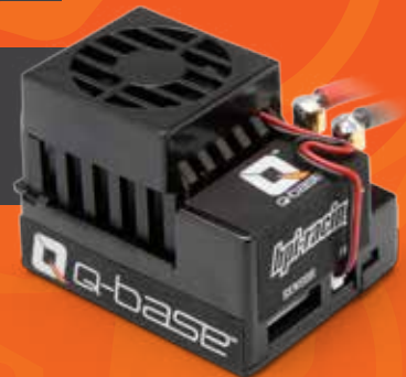
#104924 - FLUX Q-BASE BRUSHLESS ESC Compatible with sensed and sensorless brushless motor
