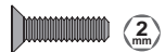
Z084 Flat Head Screw M3x12mm Senkkopfschraube M3x12mm Vis tête plate M3x12mm サラネジ M3x12mm
