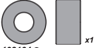
102164 Aluminum Collar 5x12x7mm (Gunmetal) Aluminium Spacer 5x12x7mm (Gunmetal) Bague aluminium 5x12x7mm (bronze) アルミカラー 5x12x7mm (ガンメタル)
